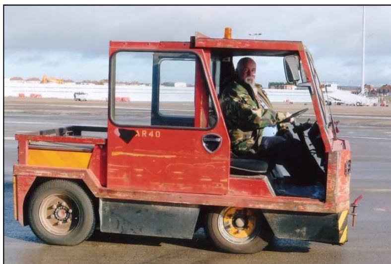
Filton's Lancing electric truck used to tow aircraft
